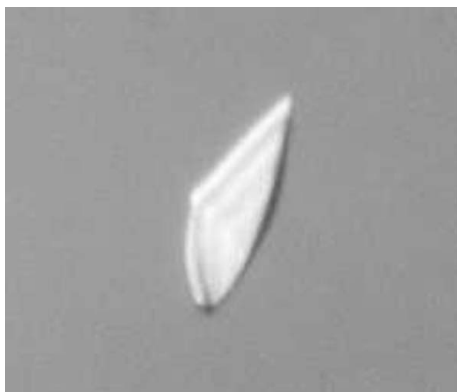
Figure 2 Crystal of the CeNA-containing octamer GTGTACAC obtained by hanging-drop vapour diffusion. The dimensions of the crystal are 0.15 \times 0.06 \times 0.06 mm.
